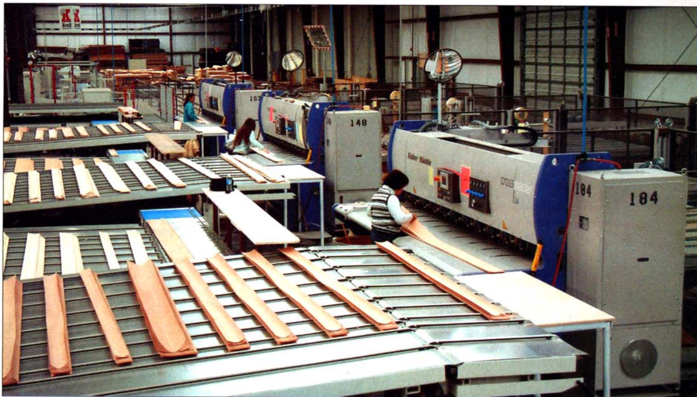
Conveyors deliver veneer to one of four Fisher+Ruckle Crossmaster splicers.
