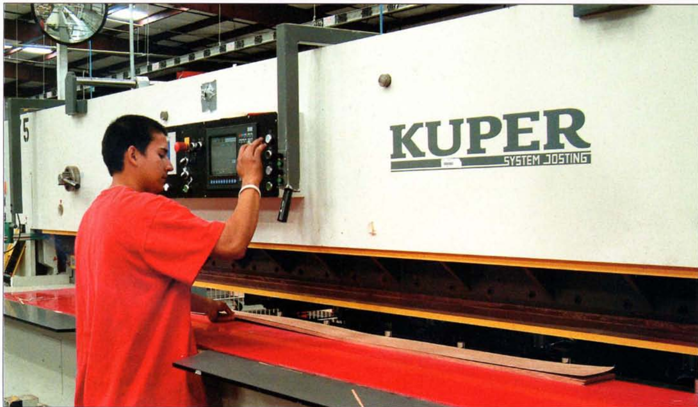
Kuper Josting double jointer operator clips veneer and inputs downstream splicer destination for each bundle.
